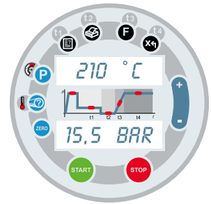
Control Display of STH TraceWeld® Hydraulic Unit
